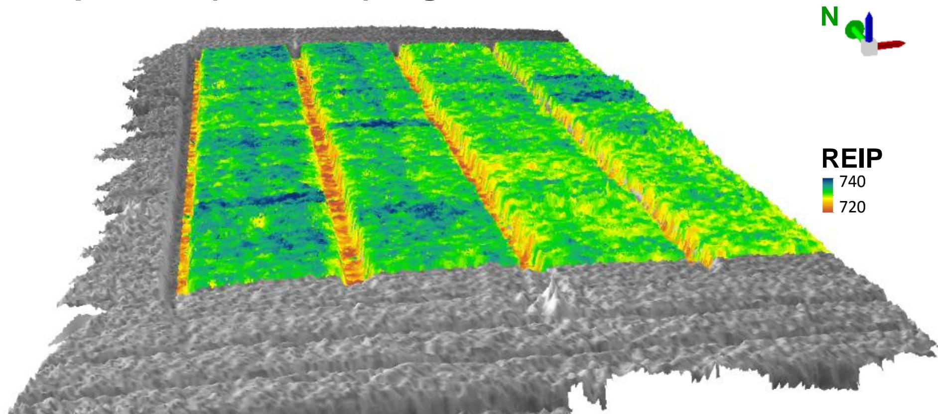
A **spectral digital surface model** is a representation of the surface in 3D space linked with spectral information emitted and reflected by the objects covered by the surface
